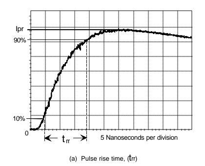
Figure 3: HBM current waveform through a 500 ohm resistor \*
