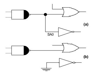
Figure <u>1</u>: (a) Fan-out Logic. (b) Same Logic with SA0.
