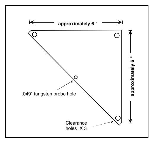
Figure A3: Top Insulating Plate
