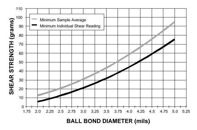
Figure 4: Minimum acceptable individual and sample average ball bond shear values \*, see Table 1 for exact ball bond shear values \*
