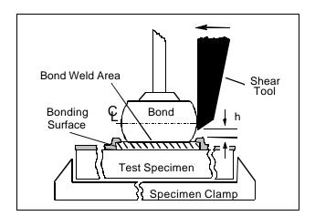
Figure 1: Bond Shear set-up
