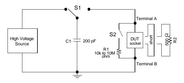
Figure 1: Typical Equivalent MM ESD Circuit
