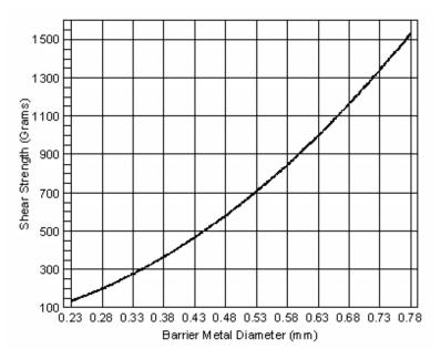
Figure 3: Minimum Shear Strength
