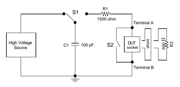
Figure 1: Typical Equivalent HBM ESD Circuit
