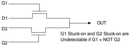
Figure 5: Wired Junction Configuration
