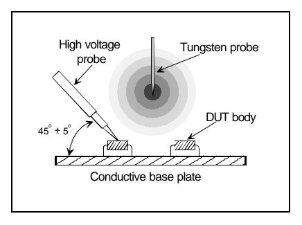
Figure 2: Measurement Angle Used to Monitor E-field Voltage
