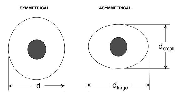
Figure 2: Ball bond diameter measurement (symmetrical vs. asymmetrical)
