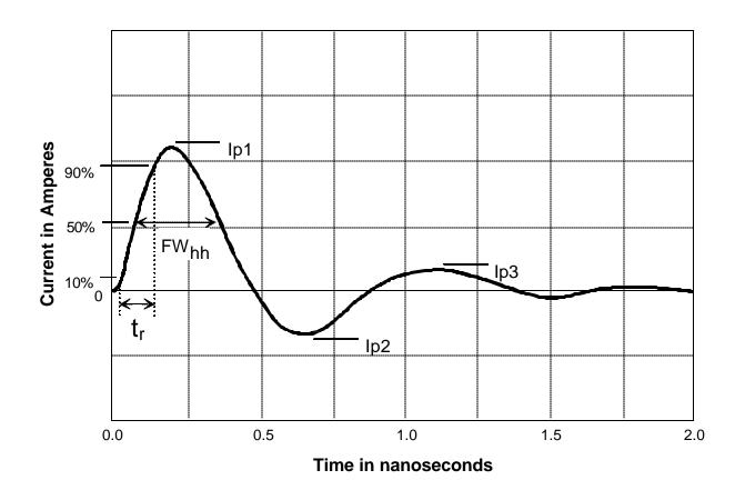
Figure 3: Typical CDM current waveform
