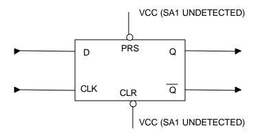
Figure 9: Power Supply and Ground Fault
