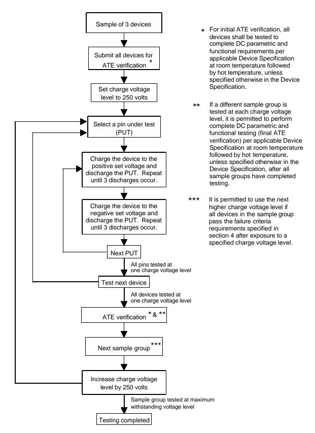
Figure 4: Integrated circuit CDM ESD test flow diagram Page 11 of 12
