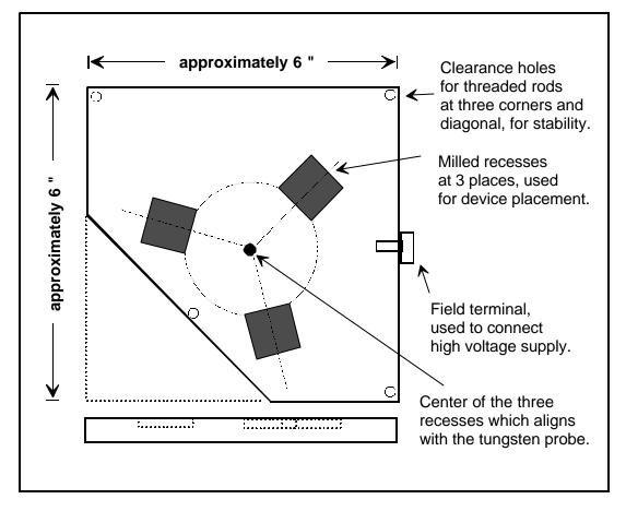
Figure A2: Conductive Base Plate
