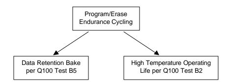
Figure 1: Test Sequence for Devices Containing NVM
